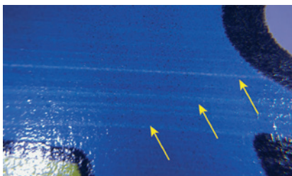
Clogged or defective print head nozzles
